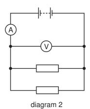
What are the ammeter and voltmeter readings in the circuit shown in diagram 2?
